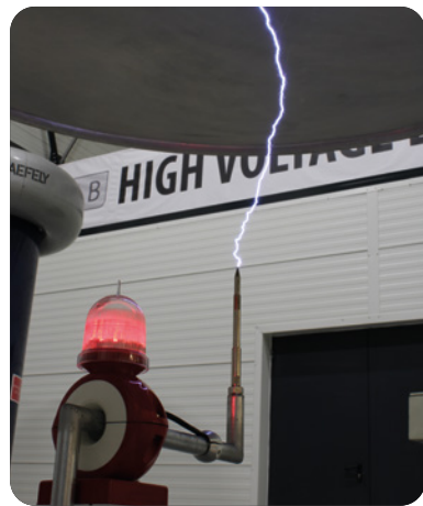
RESISTANCE TEST TO LIGHTNING STRIKES
